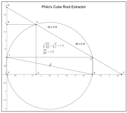
Construct a rectangle OZ with sides  $\frac{TE}{EZ} = \frac{N}{1}$  . Draw a circle with center at mid point K of TE and passing through Z. Place a ruler to pivot about point Z and adjust its so that GH=DZ. The coordinates of point H will then be the means between the coordinates of point Z. i.e., TZ : CH = CH : BH = BH : ZE
