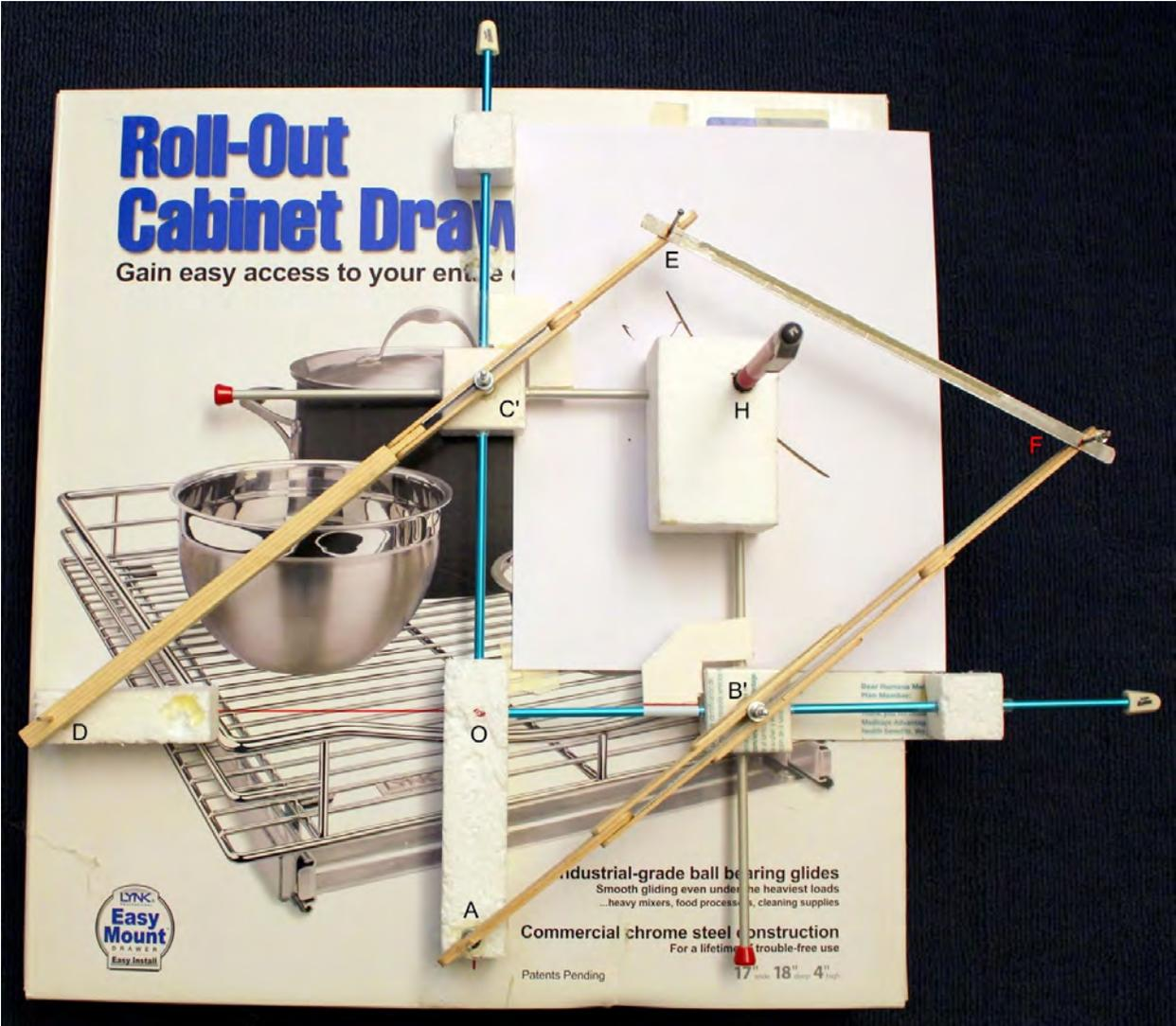
For the second curve drawn with pen L the device was reconfigured without lines AF, JB', B'H and JM and the curve was then drawn on the same sheet of paper. That configuration is not shown here.
