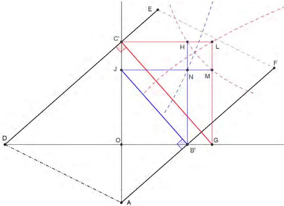
$C'$  is constrained to move along both DE and AO extended while  $B'$  is constrained to move along AF and DO extended as the sides of the parallelogram rotate while J and G are constrained to move along AO and DO extended as  $B'$  and  $C'$  move.
