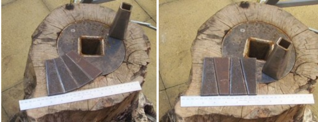
Figure 20 a,b - Tapered stake socket - sometimes it's simpler to cut each side from a parallel strip
