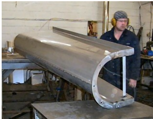
† Figure 15 - D&D Engineering Ltd. fabricate an oblique U shaped channel from 3mm thick stainless steel plate
