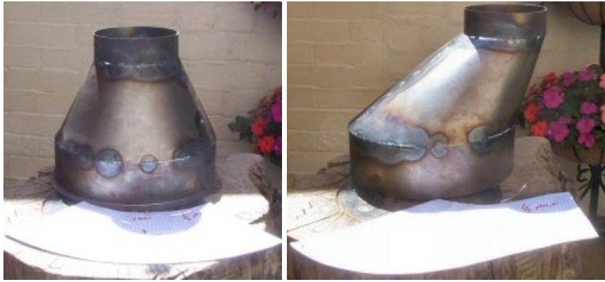
Figure 10 a,b - A right cone (parallel cuts - producing a circular input and output) and an oblique cone (which also has a circular input and output)
