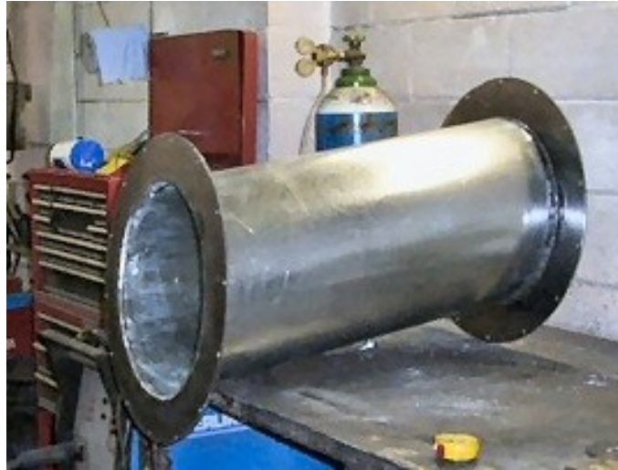
† Figure 14 - D&D Engineering Ltd. fabricate an oblique cylinder from 1.6 mm thick steel sheet
