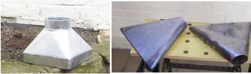
Figure 3 - Hopper for rain water guttering made from 3 mm galvanized mild steel and 2 thin sheet fan nozzles where the area of the rectangle equals the area of the circle.
