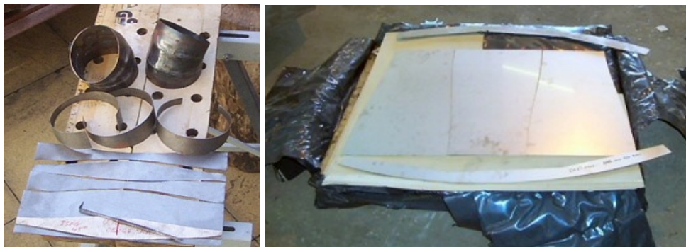
Figure 7a,b - Oblique segmental bend. Left: hand cut with shears Right: †Laser cut profiles.
