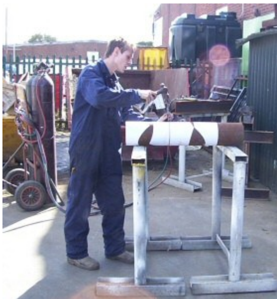
† Figure 5 – Using paper templates to mark a cutting line.
